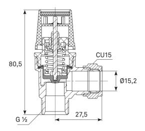
The Termoventiler SV is a safety valve for drinking water applications.
