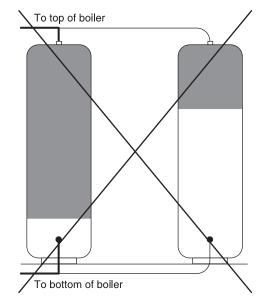
There will be imbalance between the tanks if the distance is large and/or the pipes used are too small.
