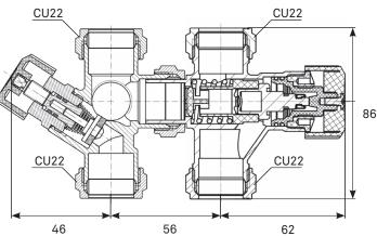
The Termoventiler VC is a combination of shut-off check valve and mixing valve for mixing tap warm water.
